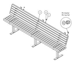
Place battens on back. Lightly tap bolts through battens and secure using hexagon dome capped nuts and M6 washers.
