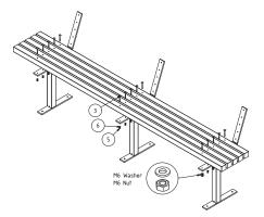
Place battens on legs. Lightly tap bolts through battens with hammer then secure using M6 nuts and M6 washers
