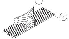
STEP 1: Place Legs (1) apart on ground. Screw bugle batten screws (3) through 50x50 profile (2) until the point shows through other side. Align with pre drilled holes in leg. Tighten screw down being carefull not to over tighten.
